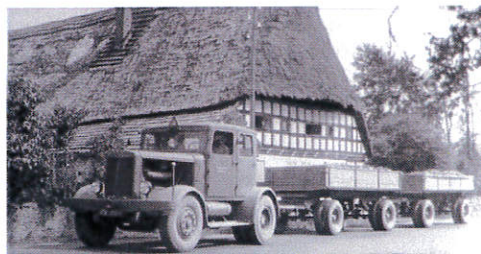
Hanomag Gigant SS100 4x2 heavy tractor - 4-doors version
