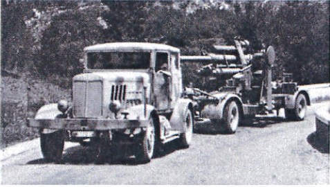
SS100 as artillery tractor, towing a 88mm AA/AT gun
